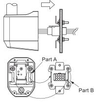
① Lower the bracket downword, pressing the bracket toward the wall.
