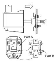
4 Lower the bracket downword, pressing the bracket toward the wall. (The installation angle is caught on the chassis of the bracket.)
