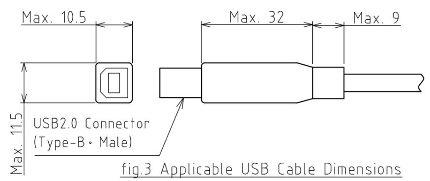
fig.3 Applicable USB Cable Dimensions
