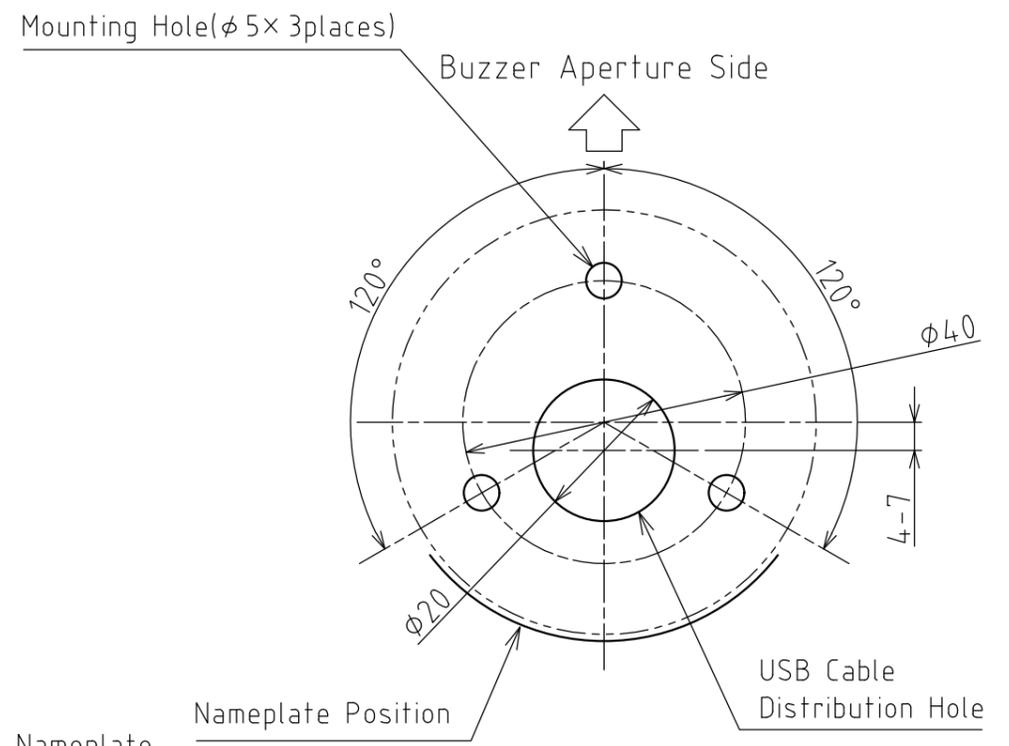
fig.2 Mounting Dimensional Drawing
