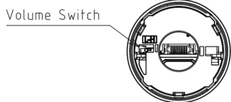
fig.4 Removed Head Cover
